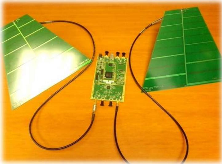
Figure 4: Indicative deployment of USRP device with two antennas
